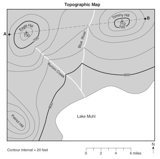
5. On the grid below, construct a topographic profile along line *AB* by plotting an **X** for the elevation of each contour line that crosses line *AB*. Connect the plotted **X**s with a smooth, curved line to complete the profile. Points *A* and *B* have been plotted.
